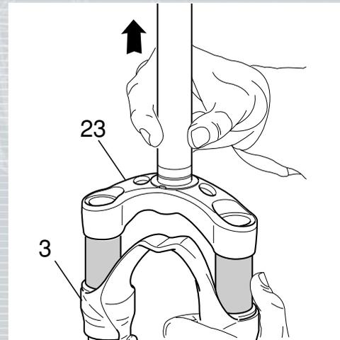
**REMOVING GUIDE BUSHING AND SEAL ASSEMBLY**
