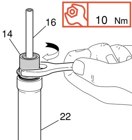
**PILOT BUSHING AND SEAL ASSEMBLY**
