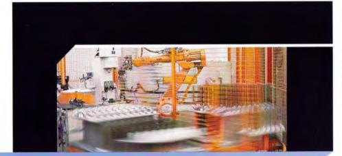
Our robotic machine has been working overtime to give every fork that precise fit by first checking every stanchion for exact tolerances, then dipping it into liquid nitrogen to cool and shrink the tube.
