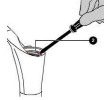
Protect the upper part of the slider with the special tool (**A**). With a screwdriver, prize off the sealing ring (**3**). Remove the sealing ring (**3**).
