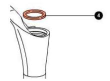
The old sealing rings and dust seals must not be used again.
