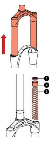
Insert spring (3), the preload tube (2) and washer (1) in the left leg.
