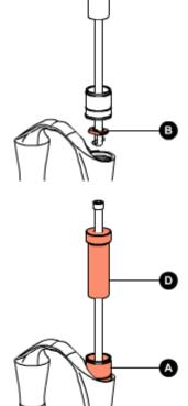
Pull the extractor rod so that the upper face of the washer stops against the lower face of the guide bush. Insert the aluminium bush (A) in the seat of the sealing ring.
