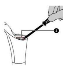
Protect the upper part of the slider with the special tool (**A**). With a screwdriver, prize off the sealing ring (**3**).
