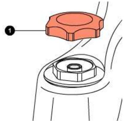
Using a small pin screwdriver, blow the air off the fork leg, pushing on the air valve.
