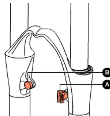
The brake cable must never touch the crown and stanchions.
