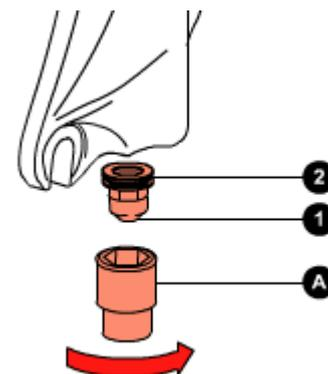
Using introducer (A) insert the dust seals (11) in their seats.
