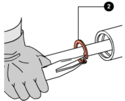
Fit the bottom pad (1) to the pumping element rod.
