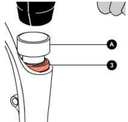
Using a small flat-tip screwdriver, fit the stop ring (2) and check that it fits perfectly into its groove. **Take great care not to damage the internal surfaces of the one-piece assembly when fitting the stop ring.** The dust seals shall be refitted when reassembling the crown-stanchion unit / arch-slider assembly.
