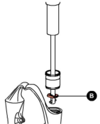
Pull the extractor rod so that the upper face of the washer stops against the lower face of the guide bush.
