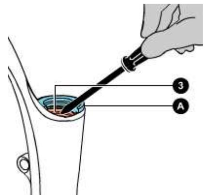
**The old sealing rings and dust seals must not be used again.**
