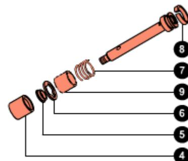
If the piston segment (8) is damaged, you can prize it off with a small flat-tip screwdriver.
