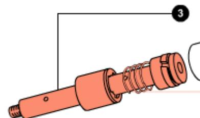
Remove bushing (4), the preload tube (9) (*only for models with 105mm travel*) and the rebound spring (7) from the pumping element.
