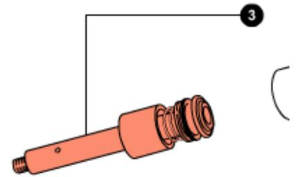
**Take great care not to damage the segment and if necessary use a small flat-tip screwdriver to help the piston of the pumping element into the stanchion.**
