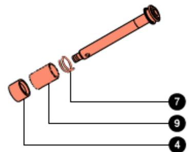
Insert the bushing in the piston rod through the hole with smaller diameter.
