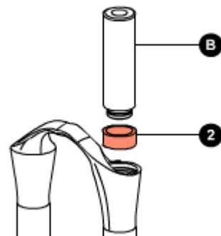
Using a hammer knock the introducer (B) into the arch-slider assembly.
