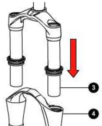
Fit washer (6) and O-ring (7) on the bottom screw (5) of both legs, then tighten to the recommended tightening torque (**10 Nm ± 1**) with the 5mm Allen wrench.
