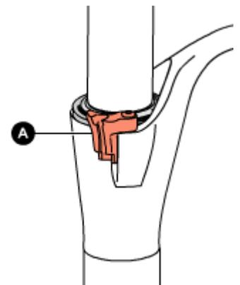
**The brake cable must never touch the crown and stanchions.**
