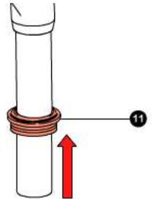
Insert the crown-stanchion unit (3) in the arch-slider assembly (4).
