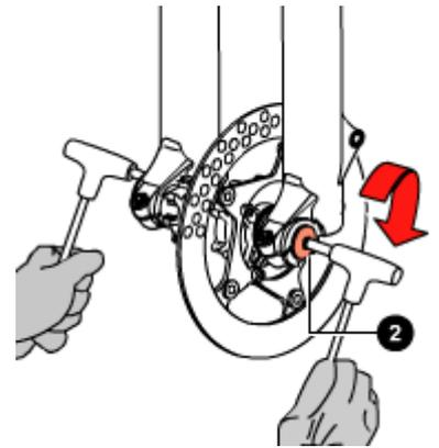
With a 4mm Allen wrench, tighten the screws (3) on both dropouts to the recommended tightening torque (**6 Nm  $\pm$  1**).
