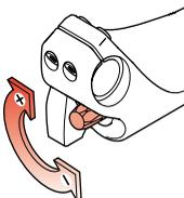
By turning the adjuster clockwise, you increase the hydraulic damping during the compression phase.
