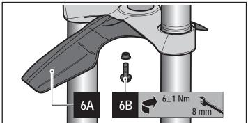
Picture 6 - Fender installation
