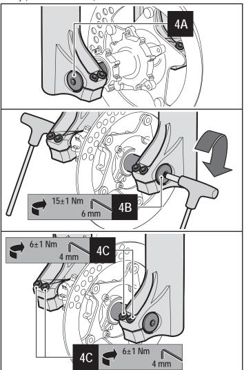
Picture 4 - Wheel install on ø35/ø38 forks with a 20 mm diameter through hole axle
