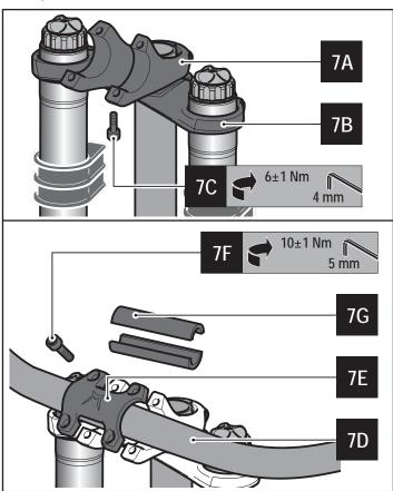
Picture 7 - Handlebar clamp installation
